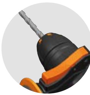
**The QS-HAMMER quick-change head** is fitted with an arrestable system for SDS-plus drilling and chiselling accessories. The fitting (arresting) and removing (releasing) of the drill bit can be done easily with one hand. The drilling depth can be readily adjusted using a large adjustment button with a depth stop located on the detachable **SOFTGRIP** handle.
